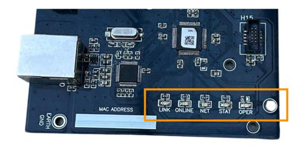
Note: View shows IP end of panel with LEDs highlighted
