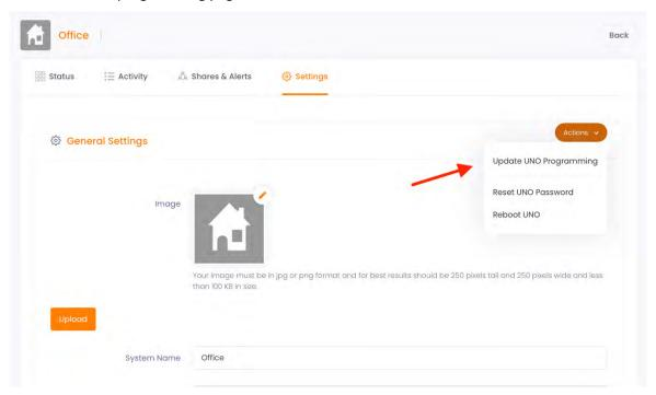
Click on "Update UNO Programming" to go to the programming section screen. From here you can choose which programming section you would like to work on. There are currently four sections; Zones, Users, FOBs, and Options.
