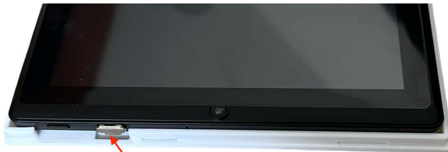
Slim USB-C connector in place. Will be hidden once cover is on.
